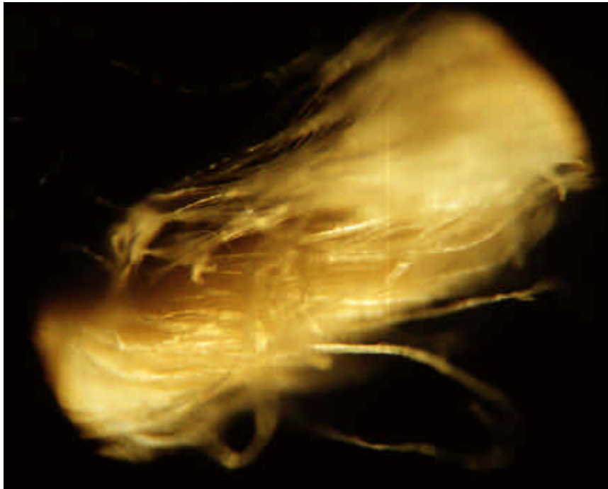
Figure 1: 100X photomicrograph taken by STURP chemist Dr. Ray Rogers demonstrating a splice in one of the threads from the Raes sample adjacent to the C-14 sample.
