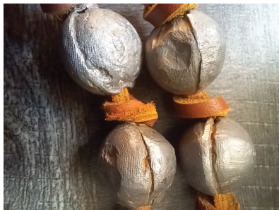
Fig. 8a. Spheres show cotton weave imprint.
