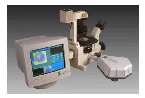
With our device, we do the reverse. Spectral imaging separates out all the colors at each point in the image. The various substances that absorb and reflect light at a specific wavelength can be determined, allowing precise, non-destructive analysis of the tissue. So if we have a protein such as hemoglobin or albumen, or if we have materials like cellulose, we can in fact understand those spectral patterns.
