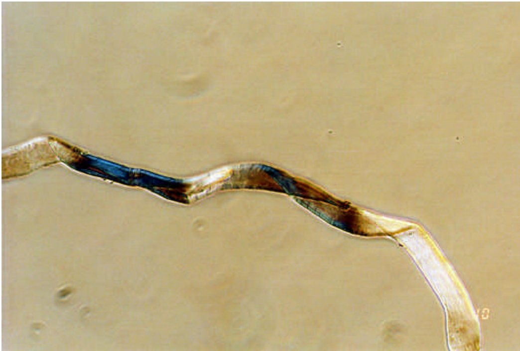
Figure 4. Cotton fiber removed from frayed end of Raes thread R14. 315X Magnification
