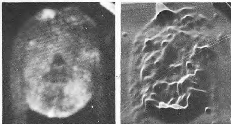
Figure 27. Engraving. Moderate Heating—No Oxide Formation.
