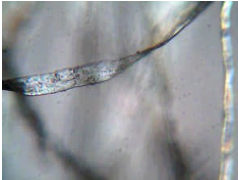
Fig.4: R7A4. Top: Low resolution: all the white fibers are cotton, while the fibers on the right are flax. The two groups are partially mixed. Middle: High resolution showing clearly cotton. Bottom: very high resolution photograph showing one of the cotton fibers with one reversal.
