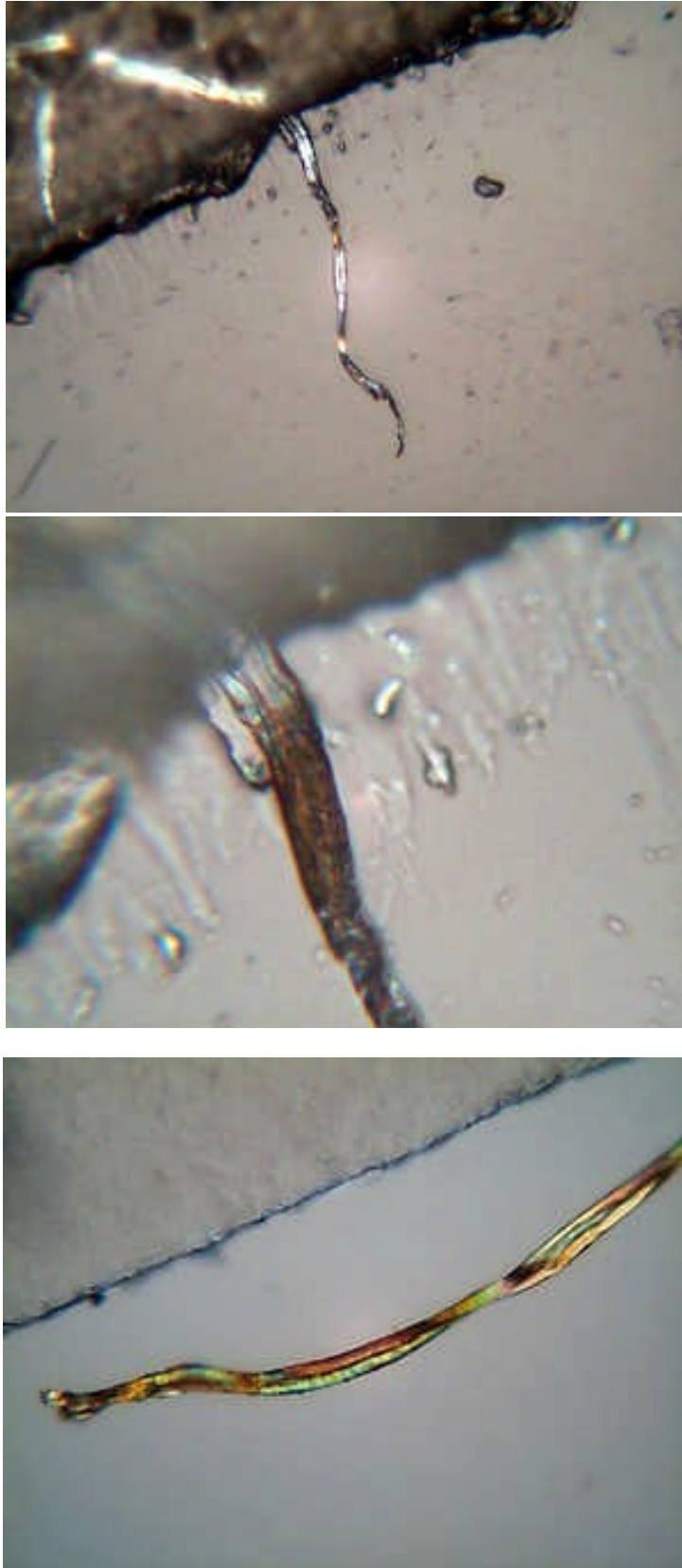
Fig.3: R7A3. Top: small piece of cotton fiber. Middle: part of the same fiber showing the typical features of cotton. Bottom: modern cotton (contamination) found in R7A3. The difference is obvious.
