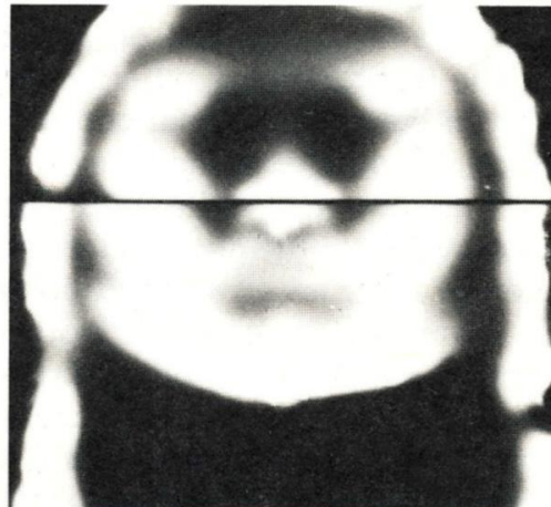
Fig. 11: Experimental radiation image with moderate attenuation between face and simulated cloth surface.
