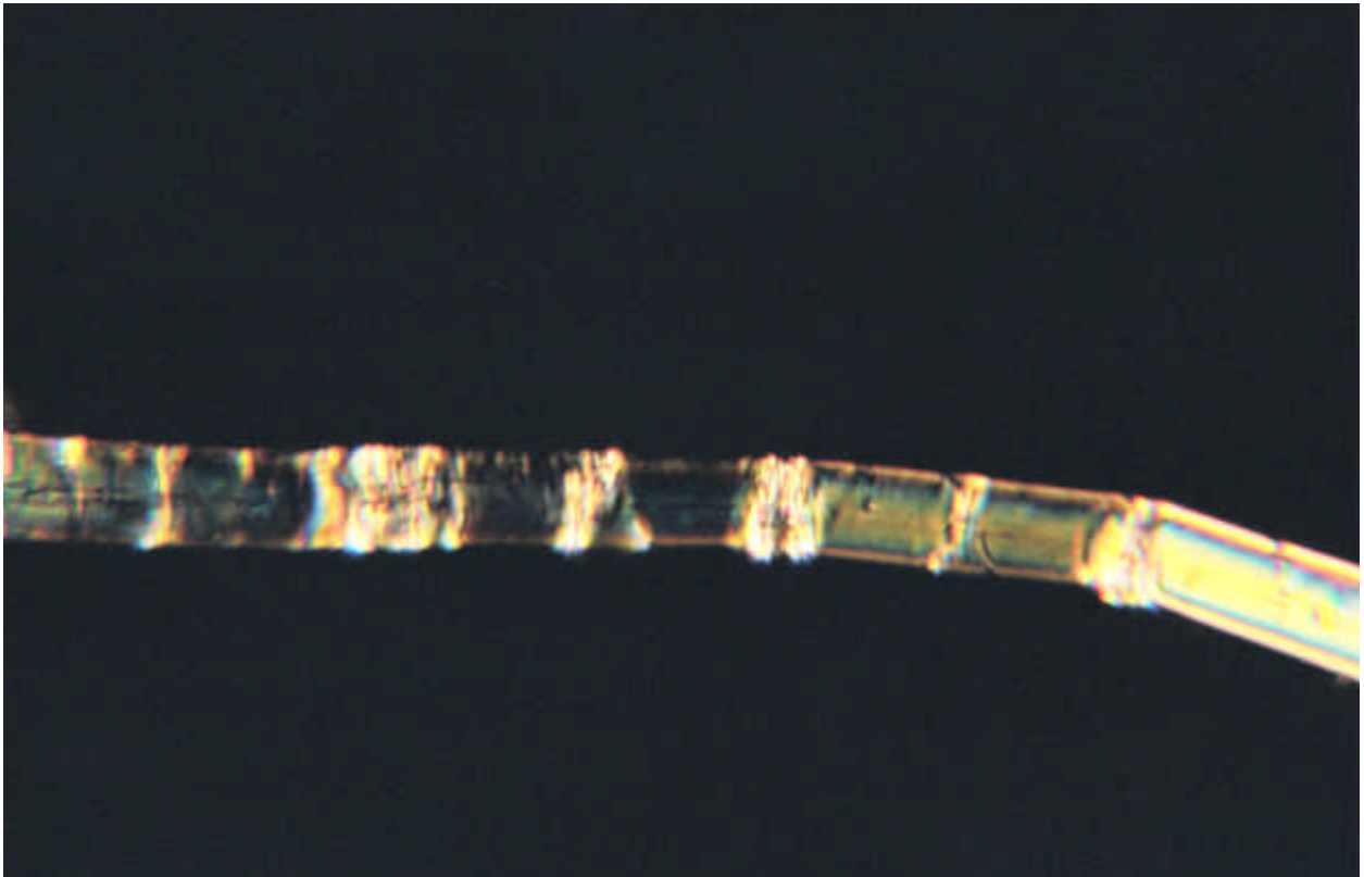
Figure 4: Flax fiber from ca. 2000 BC, 800X, polarized. It shows many dark defects, and it is quite inhomogeneous.
