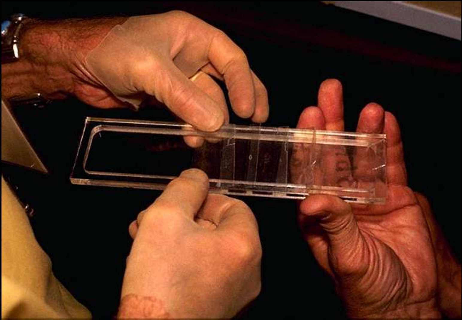
Custom well slides were fabricated to secure the tape samples by the edges and prevent any lifted debris from being embedded in the gum
