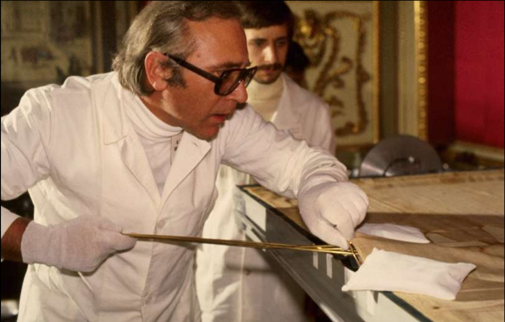
Prof. Riggi uses a custom made 'bridge' to hold the Shroud and Holland Cloth apart so the vacuum & endoscopic camera systems could be inserted between
