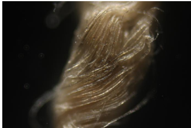
Fig. 21.- Spot isolated of black fibers in a chunk of thread of the Shroud.
