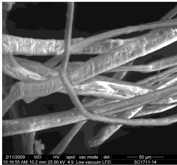
Fig. 26.- Image of fibers spotted with oxide of iron with LFD
