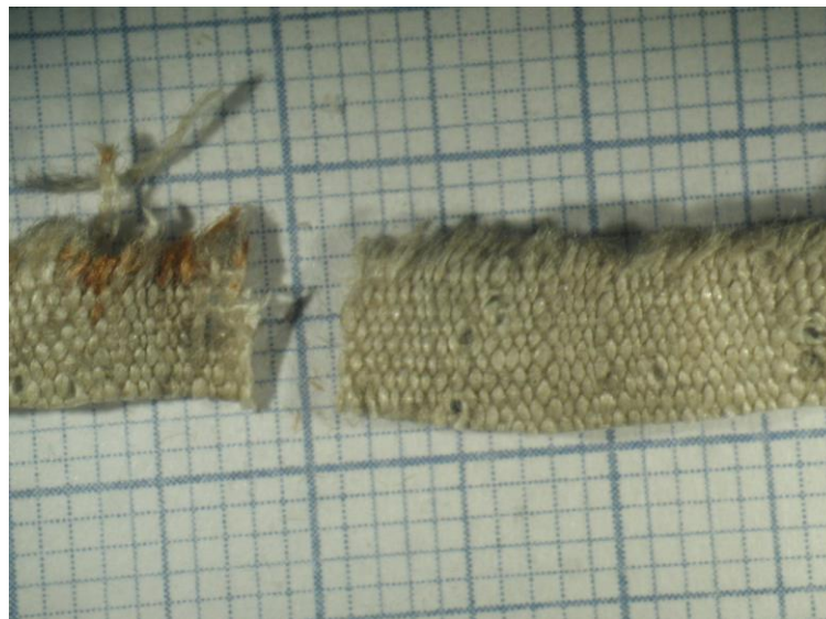
Fig. 5.- The cut sample once divided to eliminate the zone contaminated by oxides of iron.
