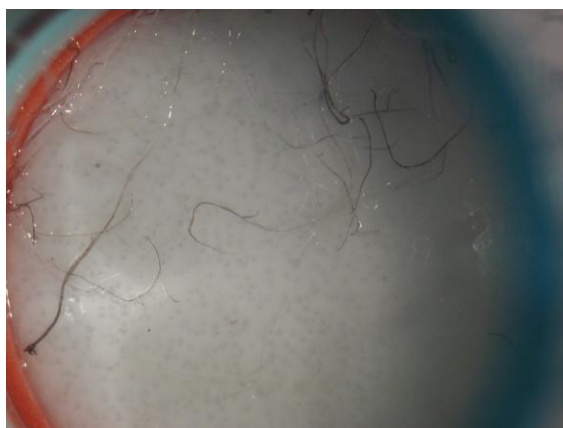
Fig. 41.- Black fibers after the previous treatment used by BETA ANAYTIC.
