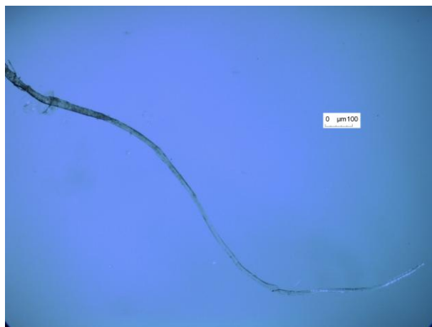
Fig. 34.- Black fiber showing a black zone and the clean rest.
