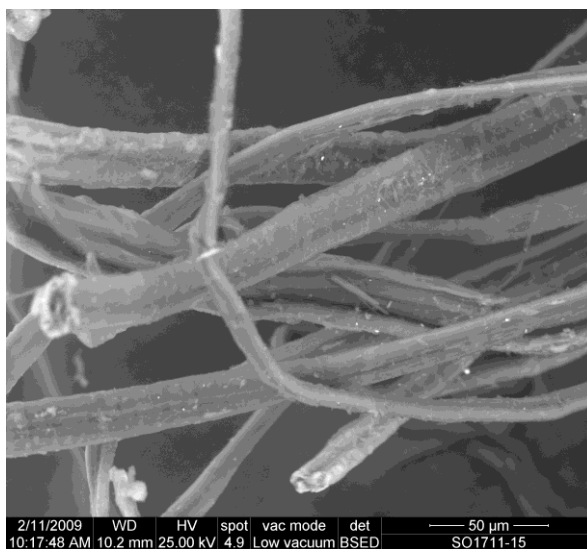
Fig. 27.- Image of fibers spotted with oxide of iron with BSED.
