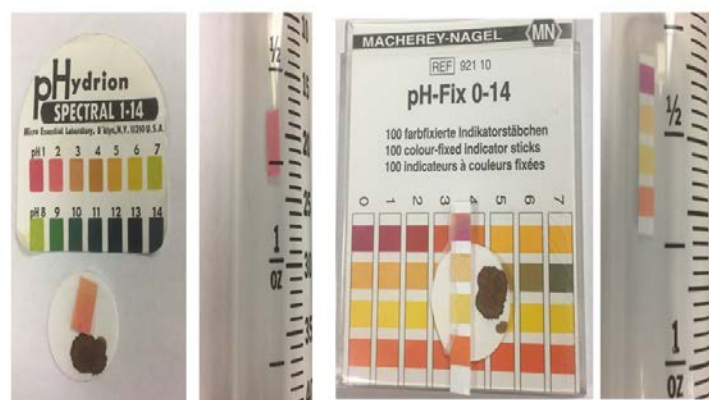
Figure 4. Generation of products in the reaction mixture results in a change in pH. CO gas was generated using the acid mixture protocol and streamed over bloodstains to which two different types of pH indicator paper were attached. Additionally, pH indicator paper was included in the gas collection syringe. Upon exposure to gas, a drop in pH was observed from approximately 7 to 2-3. No pH change was observed with each reactant was singularly used in the protocol (data not shown); see text for details. The results shown are representative of at least three separate experiments.
